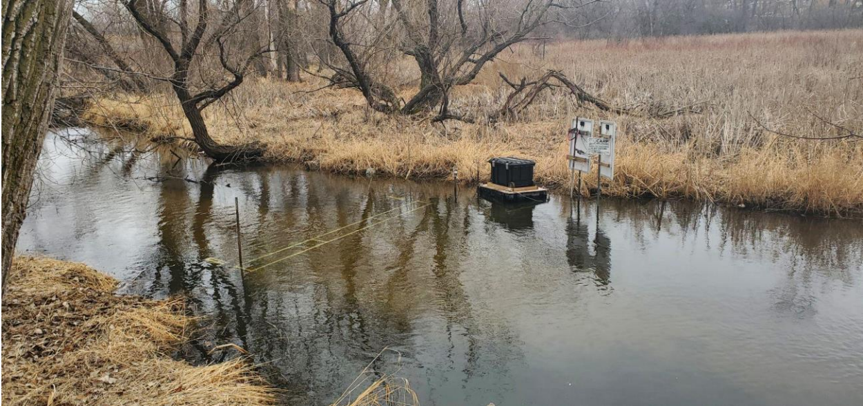
Figure 1: A PIT antenna system in a stream in Minnesota for tracking the spring migration of PIT tagged common carp.
