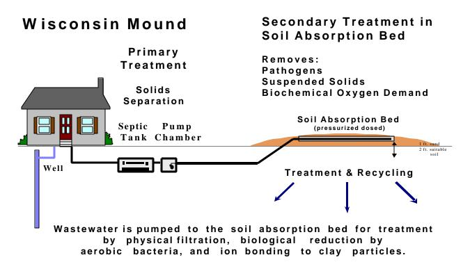
A mound system, like a conventional system, consists of a septic tank and a soil absorption bed. In the mound system, however, sand is added where suitable native soil is insufficient. Clarified effluent from the septic tank is pumped, in controlled pressurized doses, to an aboveground, freestanding sand layer. The sand layer, placed upon a specially prepared area of native soil, serves as the medium on which aerobic bacteria facilitate much of the secondary treatment.
